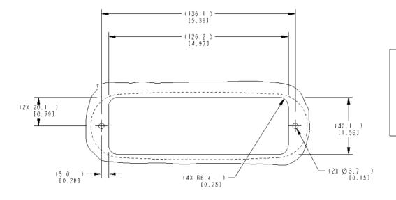
Install with 2 #8 or M4 flat head screws. Do not exceed 13.6 in-lbs torque when installing screws.
